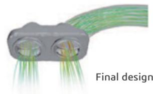
The use of TOSCA Fluid in the redesign process resulted in a pressure drop reduction of up to 50%, better flow efficiency, and overall cost savings. For an enhanced comfort, the flow distribution ratio between driver and passenger was improved from 40%/60% to almost equal.
